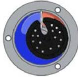
3- The liquid fills progressively the inlet measuring chamber (in red), as it is getting emptied on the outlet (in blue). In the middle of the cycle (see figure) the two chambers are the same size.
