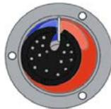
5- At the end of the cycle, the inlet measuring chamber takes all the space. From this moment it can be considered that this is already the outlet chamber, so we are again at the beginning of the cycle.
